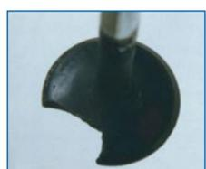
**Remedy:** Check the remaining valves for signs of cracking, replace where necessary. Ensure
