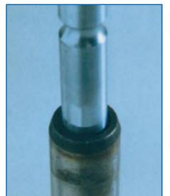
**Remedy:** Ensure correct valve and guides are fitted. Check alignment, valve stem to guide clearances, valve stem seals and lubrication system.
