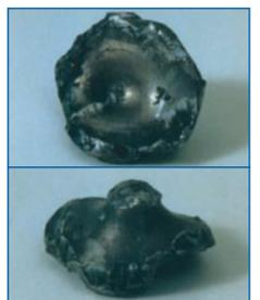
**Remedy:** May not be possible due to extreme damage this failure can cause, however: Check valve springs, guides and alignment and repair where necessary. Check seat guides, pistons and bores for damage. Reset the valve clearances.
