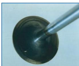
**Remedy:** Check remaining valves for signs of cracking, replace where necessary. Ensure the correct valves have been used. Check engine settings, valve springs, guides and followers. Do not overspeed engine.
