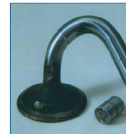
**Remedy:** May not be possible due to extreme damage this failure can cause, however: Check seats, guides, springs, pistons and bores for damage and repair where necessary. Do not overspeed the engine.
