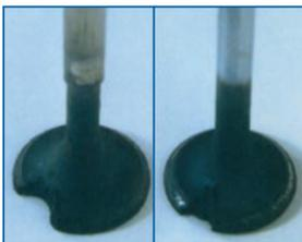
**Remedy:** Ensure valve clearance is to specification. Check stem to guide clearance and for any misalignment of the valve assembly.
