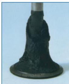
**Remedy:** Check valve stems, guides and stem seals for wear and replace where necessary. Ensure there is no blockage in the engine drainage or breathing systems.
