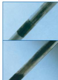
**Remedy:** Ensure the valve stem to guide clearance is to specification. Ensure the correct valve stem seals have been used. Replace worn components where necessary.
